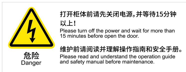
Figure 1-6 Door Power Loss &amp; Maintenance Signage
