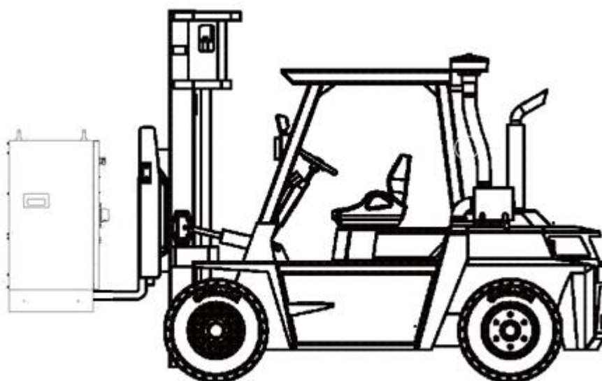
Figure 2-2: Control Cabinet – Forklift Handling
